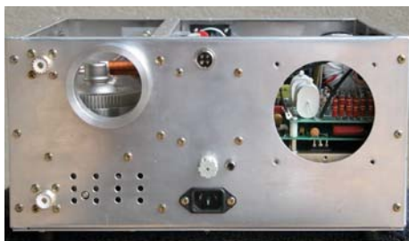
Rear view, showing RF input and output connectors at bottom left and top left. Also shows the mounting flange for the blower, cathode compartment air exhaust (under blower flange), AC power connector for blower and fan upper center, fuse, RCA PTT and AC mains connector, hole for muffin fan at far right. Both openings are 'screened' with stainless screening.
