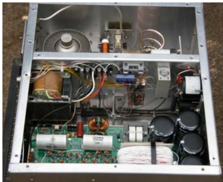
Another view of RF deck, showing the 8877. Also shows the anode clamp and input/output relay switching board, featuring the Schrack relays. Also note the Teflon RG-142 coax for the output which will handle the 1.5 kW without meltdown! Also shown is part of the control circuitry: Omron time delay relay and Tripplett 120G series plate and grid meters. The fuse at the centre is the 1 amp cathode circuit fuse.
