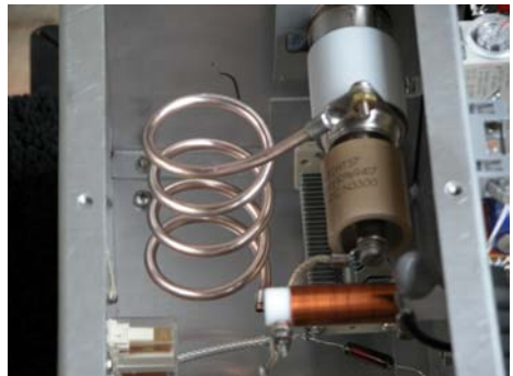
Larger view of tank circuit, showing silver-plated tank coil, 3-30 vacuum variable, 857 blocking cap, RF plate choke and almost buried at the bottom, the 200 pf loading cap.
